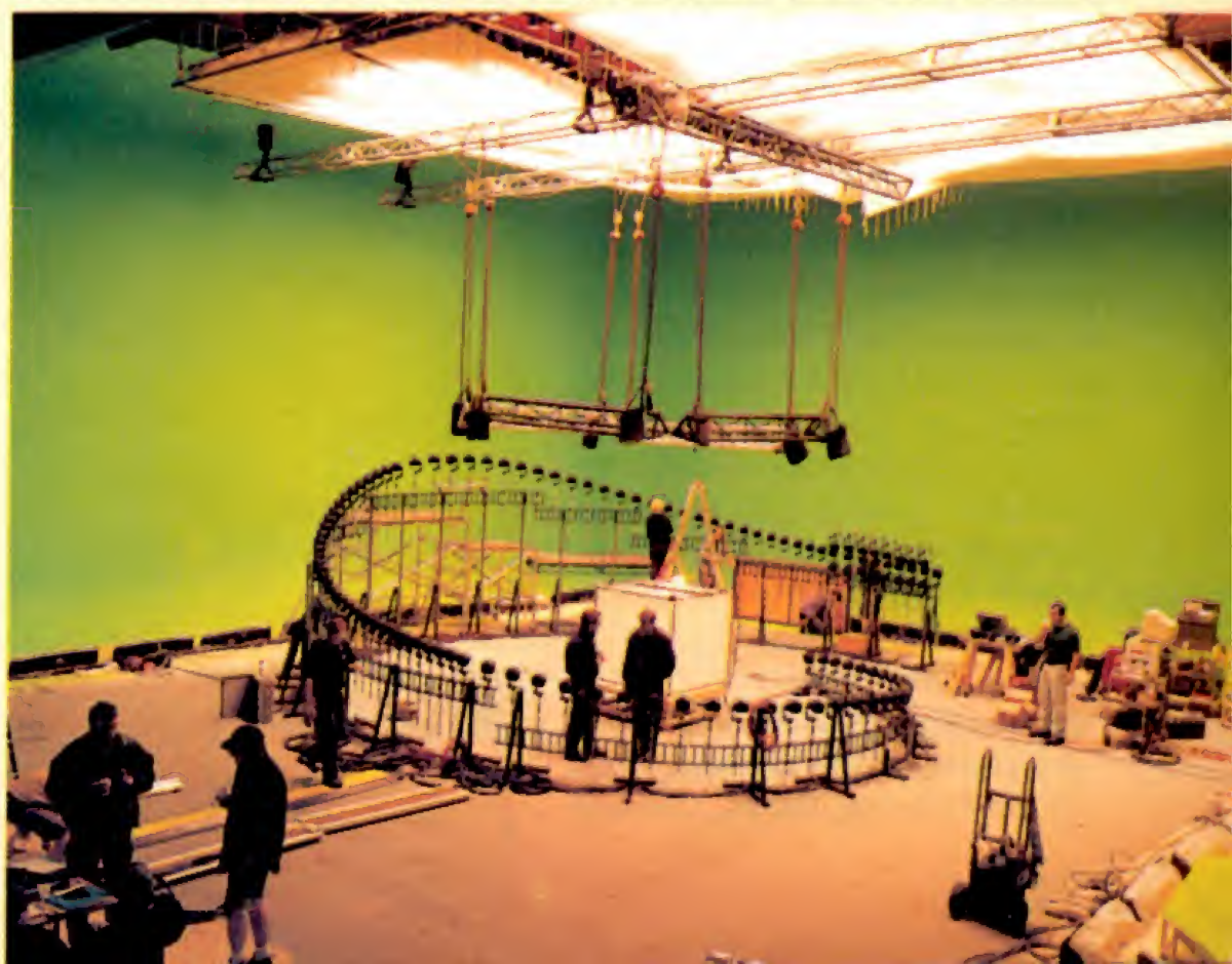
Setting up the roller coaster formation of the film's “bullet time” slow-motion still cameras, filmed green screen to composite actors and effects in real time.
